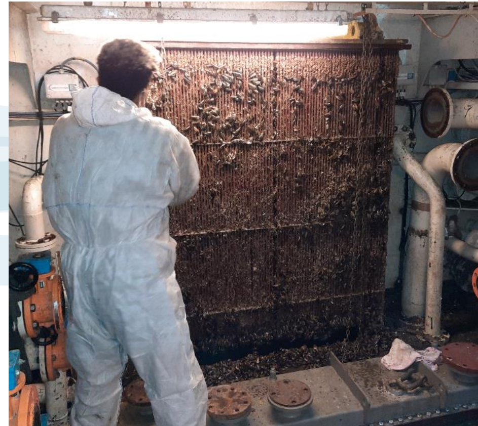
Time-consuming, heavy labour is required to clean the box cooler. This is an example and is not from a Royal IHC ship.
