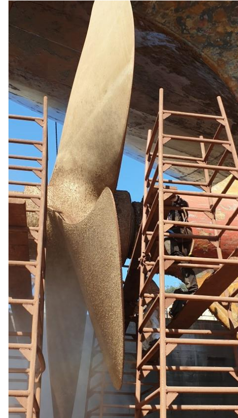
Propeller after installation Ultrasonic Anti-Fouling system
