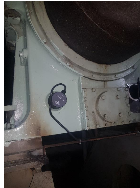
Transducers on intermediate bearing
