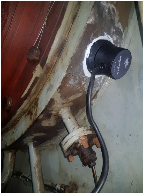
Transducers on aft stern tube bearing
