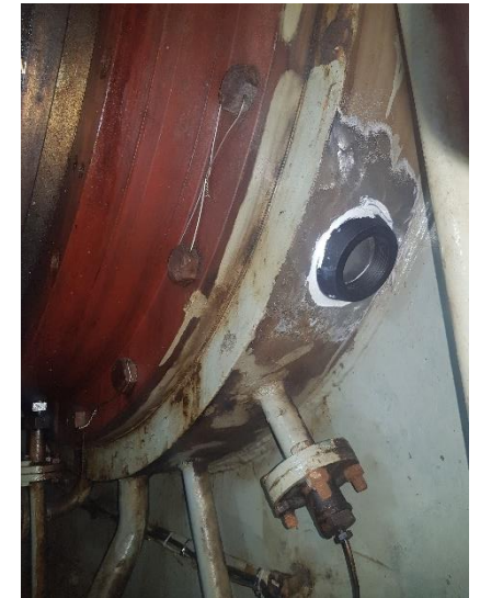
Glued transducer ring on stern tube bearing
